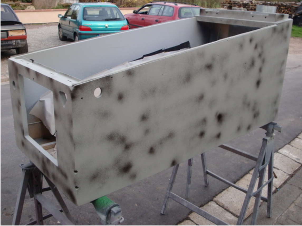
Injection plaster was applied to the casing
