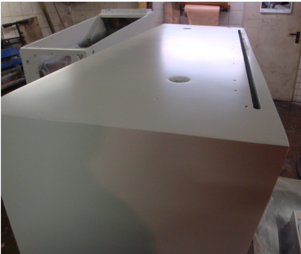
Spray filler finish polished by the housing
